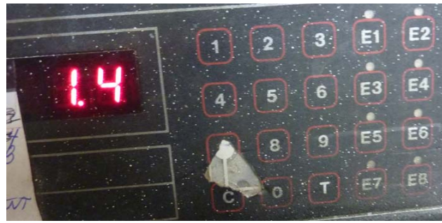
Set the exposure time by pressing keypad. Decimal is automatically inserted. Exposure time is pre determined by using a marked film positive supplied by a film positive manufacturer. A plate is cut into small rectangles that are exposed at varying times, then developed, and examined with a magnifying loop. The developer must easily dissolve out the exposed unwanted background, while leaving the small 5% highlight dot in making up the tint of the solid.
