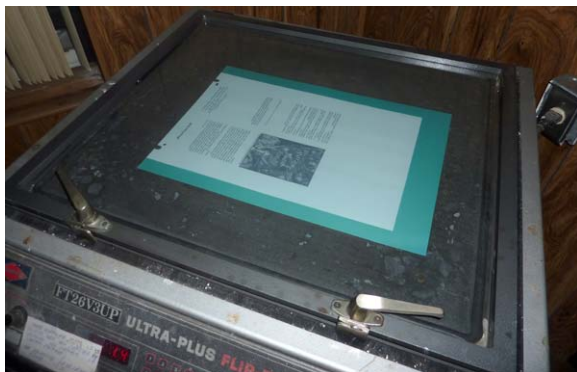
Plate & film aligned to each other by punch marks, and centered in exposure box. Image is read right looking down, but laser printed flip horizontal on underside of film so toner is closest to plate surface and distortion from thickness of film is eliminated. Two handles are locked before vacuum is turned on to eliminate air between plate and film surfaces. When maximum vacuum is reached as indicated on the gauge, the black lever on the right is pulled downward and the top of the machine is flipped 180° where it is held in position by a detent. Then the letter T on the keypad is pressed to start the exposure. When the time is up, the exposure stops.
