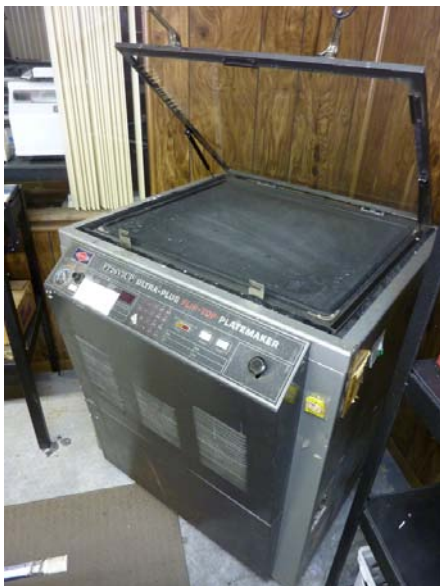
Open lid on plate exposure box. Clean glass lid inside and out. Exposure time was determined to be 1.4 units for positive plate brand I use.
