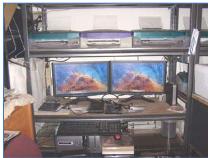
One Computer Running Ten Inkjets Through Two USB Hubs
