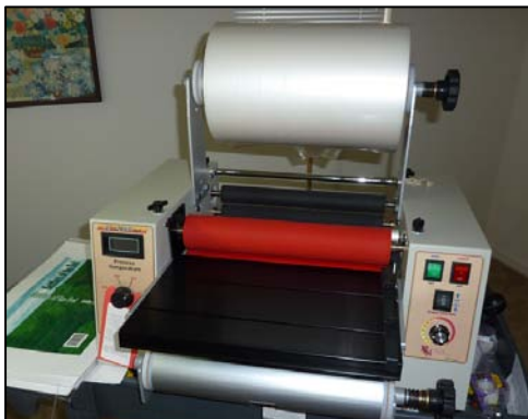
Pro Lam P1200 double sided laminator being used to put a protective .0014" thick glossy film on the outside of book covers. The heating element inside the rollers design allows for a faster feed speed at 250° less, with no annoying curl of the finished product. Film material is 11.75" wide centered on 12" x 18" digital cover stock at 10 or 12pt thickness.
