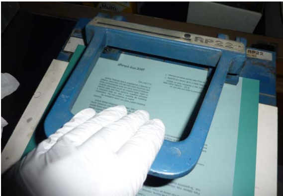
Before exposure, film image is centered side to side on the light sensitive plate, and even with the top edge of the plate. The punched holes align the plate when it is mounted on the press plate cylinder, and two additional small holes keep the film straight during exposure.
