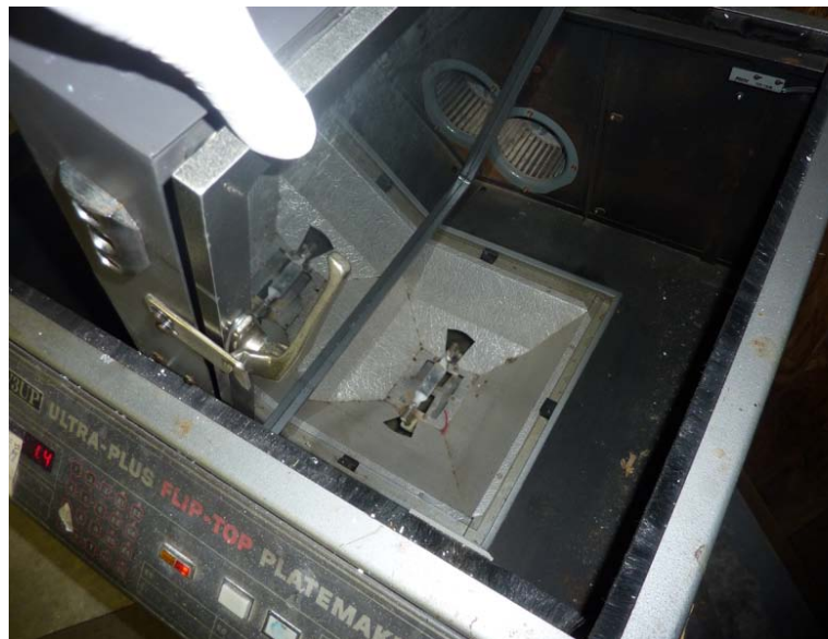
A 3000 watt mercury vapor bulb costing over $100 runs on a 220 volt electrical circuit to expose aluminum printing press plates. One must use cotton gloves when handling the bulb.
