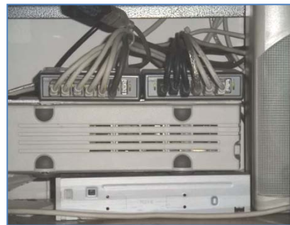
One Computer Running Ten Inkjets Through Two USB Hubs
