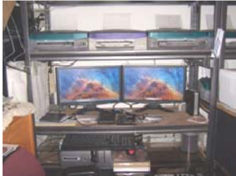
One Computer Running Ten Inkjets through Two USB Hubs
